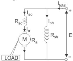
➤ When the shunt winding is so connected that it shunts the series combination of armature and series field it is called long-shunt connection.
