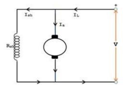
In this circuit the field winding is directly connected to the source voltage, so the field current Ish and the flux in a shunt motor are constant.
