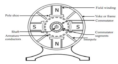
Salient parts of a D.C.Machine are:
