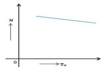
➤ The speed reduces when the load torque increases.
